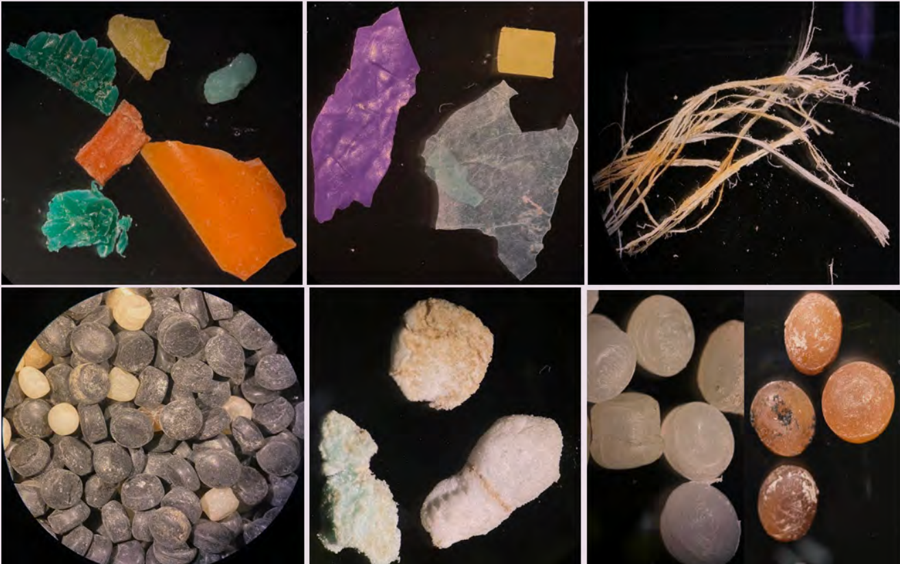
Figure 2. Different types (fragments, films, fibers, pellets and foams) of microplastic particles in beach sediments from the Ras Rakan Island.
