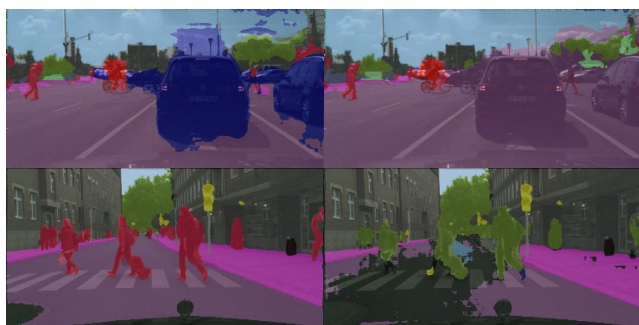
FIGURE 2. This is a presentation of two sets of local source domain attacks. In the above two pictures, we attack cars (blue) as road (pink) while the pedestrians (red) are attacked as the vegetation (green) in the below. When the source domain is a convex set, the perturbations added is easy to attack the model. But when the source domain is irregularly shaped, this attack affects the classification of adjacent pixels, especially where there are other non-target classes embedded in.
