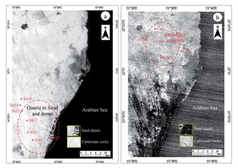
Figure 3. (a) Quartz index (QI), and (b) Carbonate index (CI) images show the occurrence of quartz and carbonate minerals as bright features. Locations represent the sites of image spectra collected over sand deposits and carbonate rocks.
