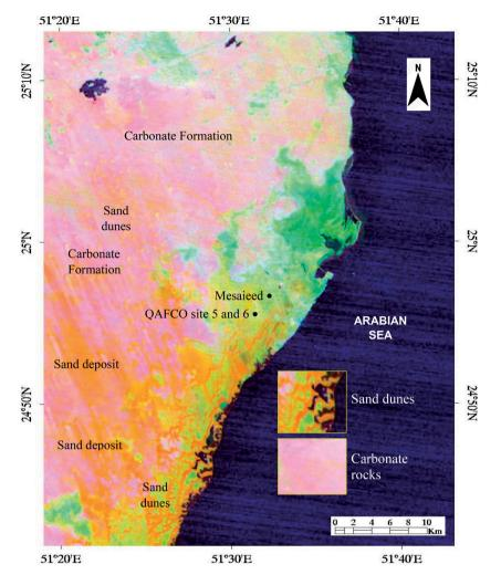
Figure 4. False-color composite (R: Band 6; G: Quartz index; B: CI index) showing the occurrence and distribution of sand deposits, dunes and carbonate formations in the east coast transect of the State of Qatar.
