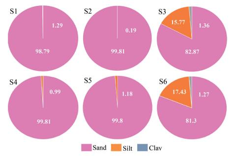
Figure 8. Distribution of sand, silt and clay in the sand deposits found in and around QAFCO site 5/6. Values are in percents.
