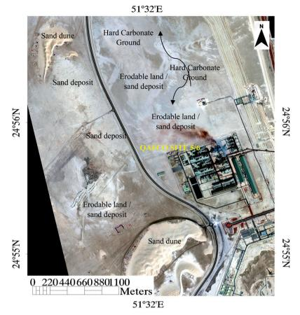
Figure 5. WorldView-2 satellite image acquired on February 16, 2021 showing the sand deposits in and around the QAFCO site 5/6.
