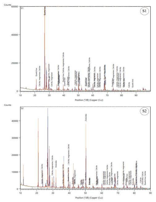
Figure 9. XRD analyses of sand deposits of QAFCO site 5/6 showing the presence of quartz, calcite, magnesian calcite, dolomite, albite (quartz silicate) and halite minerals.
