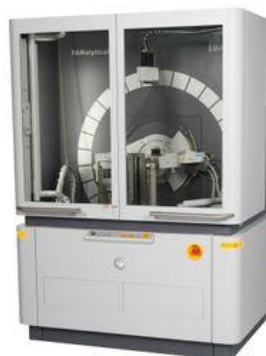
Figure 18: PANalytical Empyrean diffractometer.
