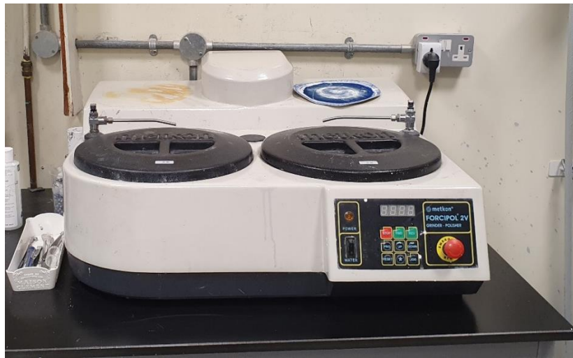
Figure 12: Metkon Forcipol 2V grinding and polishing machine.
