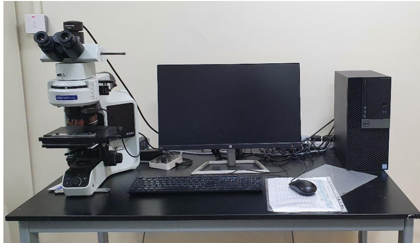
Figure 17: Olympus BX53M optical microscope.
