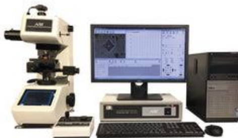
Figure 22: FM-ARS 9000 hardness testing device.
