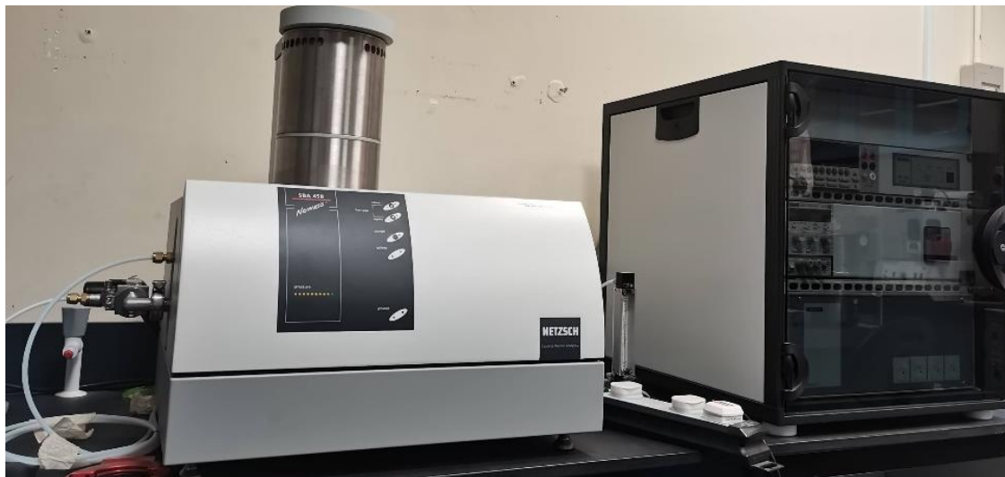
Figure 22:Electrical conductivity SBA setup(Nemesis), Qatar University
