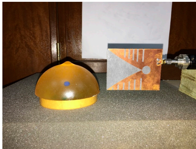
Figure 3. Reflection coefficient measurement with a phantom load.
