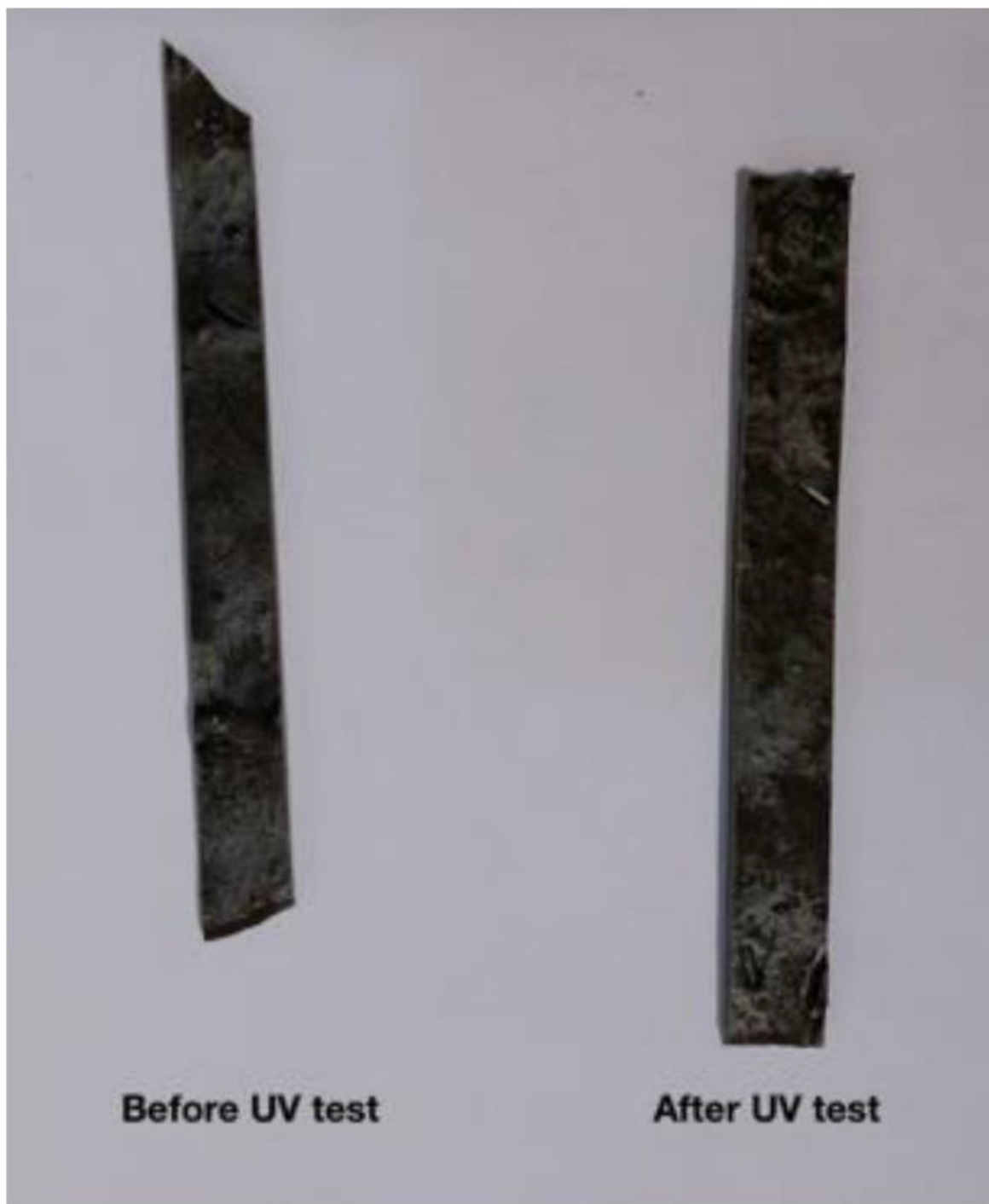
Fig 9. Changing in color pigmentation before and after UV aging test for DP0S50E.
