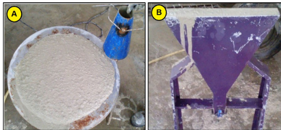
Figure 9. Experiments on fresh concrete: (A) slump flow test apparatus; and (B) V-funnel test apparatus. Reproduced from [81].
