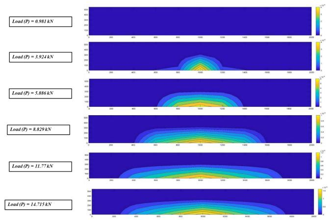
Fig. 2: Simulation of Strain Contour of One-Way Slab
