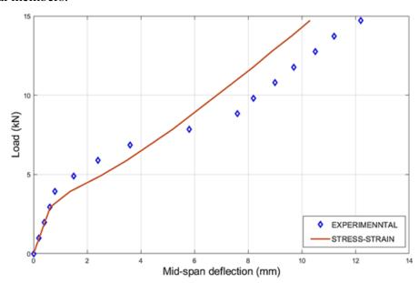
Fig. 1: Load-Deflection for a slab subjected to point load
