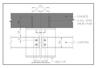
Fig. 8: Struct & Bracket (Section) (dimensions in mm)
