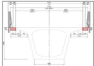
Fig. 2: Option of Extending Both Sides of the Deck (dimensions in mm)
