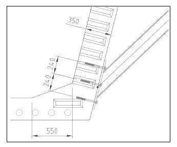
**Fig. 9:** Strut-Girder connection (Section) (dimensions in mm)
