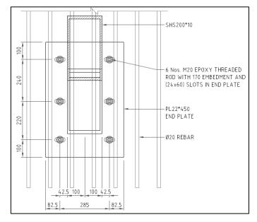
Fig. 10: Strut-Girder connection (Plate details) (dimensions in mm)
