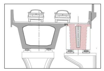
**Fig. 1:** Option of Adding a New Bridge Deck
