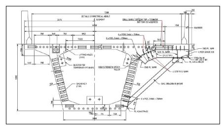
Fig. 3: Bridge Deck Cross-section (dimensions in mm)
