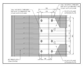
Fig. 6: Bracket (Plan view) (dimensions in mm)
