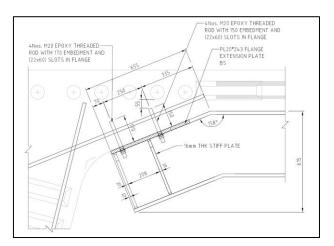
Fig. 5: Bracket (Section) (dimensions in mm)
