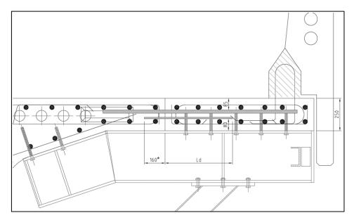
Fig. 11: Caption of Embedded Reinforcement (dimensions in mm)
