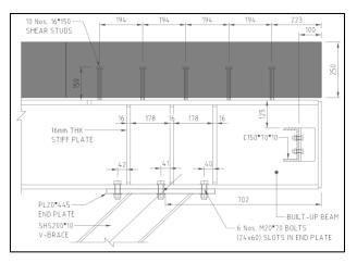
Fig. 7: Strut & Bracket (Section) (dimensions in mm)
