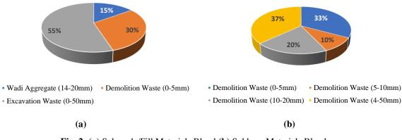
Fig. 2: (a) Subgrade/Fill Materials Blend (b) Subbase Materials Blend
