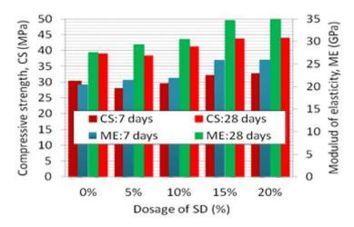
Fig. 5: Compressive strength and modulus of elasticity of SCC
