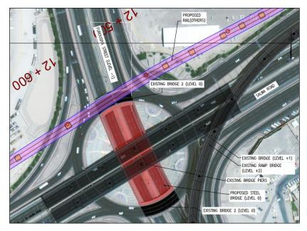
Fig: 1: Layout of Junction 101 with the existing and proposed bridges
