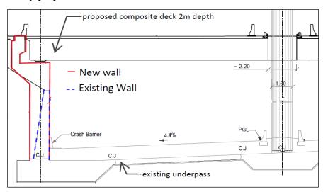
Fig. 2: Reference Design Typical Section
