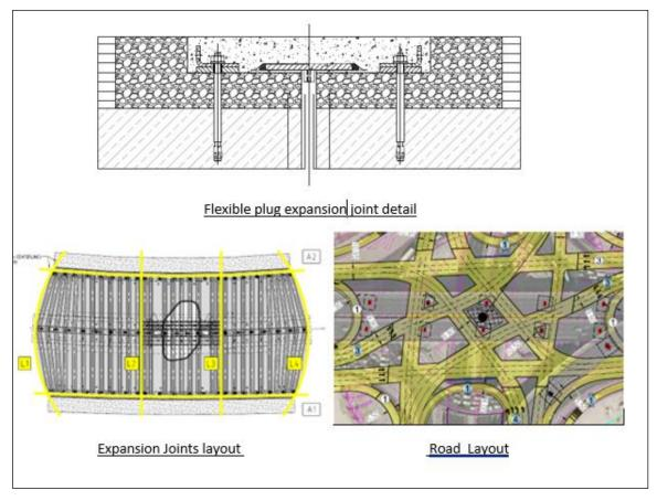
Fig. 7: Flexible plug expansion joints details and layout
