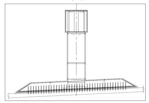
Fig. 8: Median Pier integrated footing
