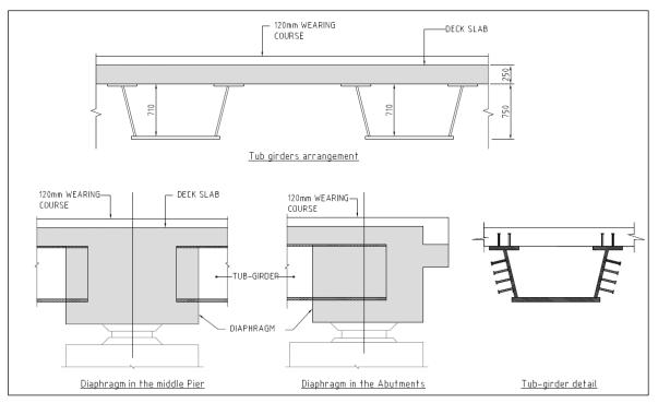
Fig. 6: Typical deck details
