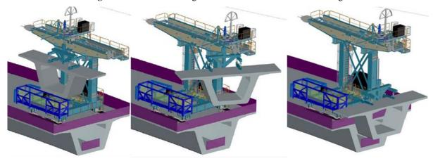
Fig. 6: Installation of Precast concrete Segments using Lifting Frame
