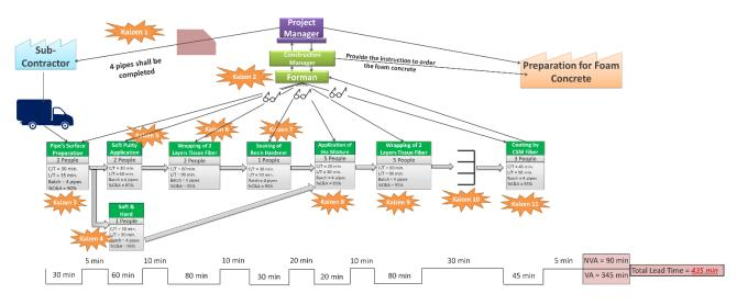
Fig. 2: Future State of Manhole's Connection Process
