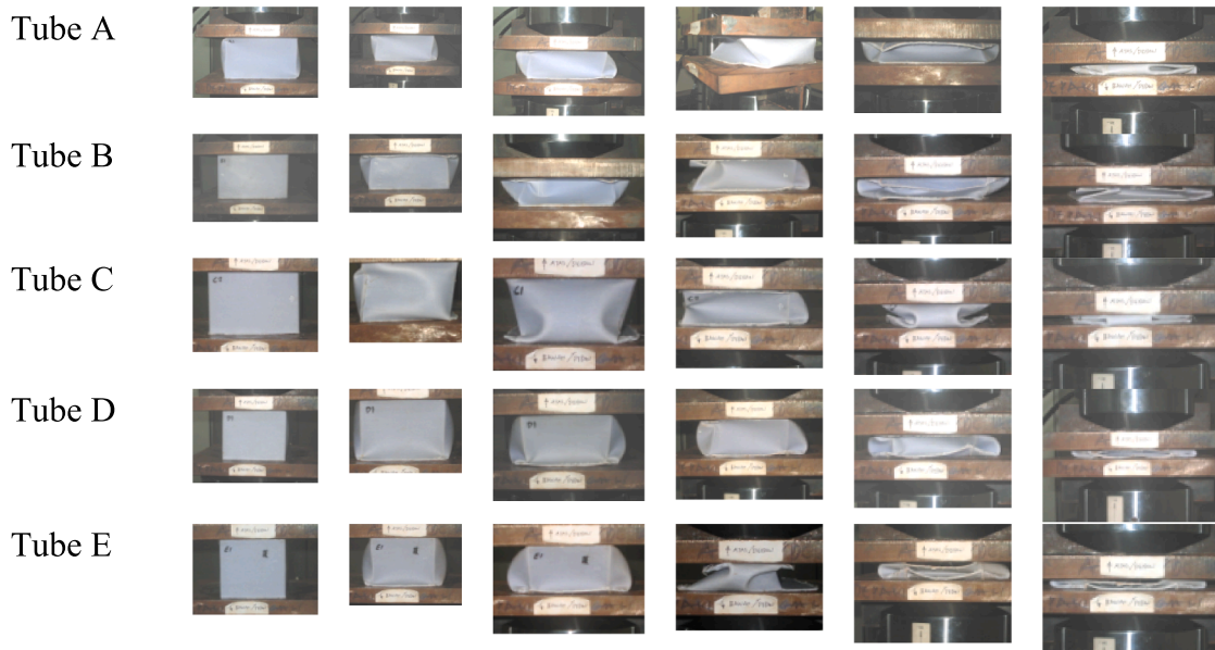
Fig. 2b. Crushing history of axially crushed tubes with different aspect ratios.
