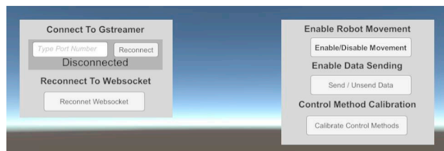
Figure 7. The graphical user interface of our system connects with Gstreamer and WebSocket server (robot control software), allows enabling/disabling the robot's movements or sending data, and for starting the calibration process of the control methods.
