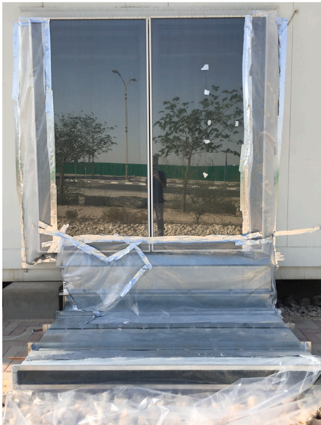
Fig. 3. The evaporatively-cooled façade system installed in the Zero Emission laboratory for experimental validation.
