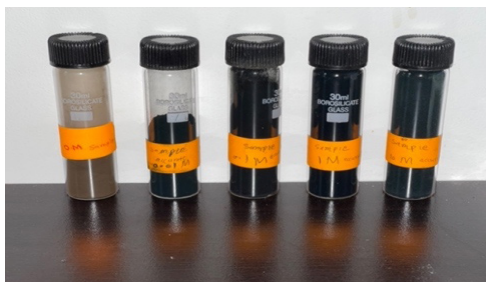
Figure 1: The physical appearance of PANI yielded using different concentrations of HCl. (Bottle arranged from left to right is for PANI produced using 0 M, 0.01 M, 0.1 M, 1 M, and 10 M of HCl).
