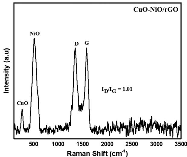
Figure 3. Raman spectrum of the prepared CuO-NiO/rGO nanocomposite.
