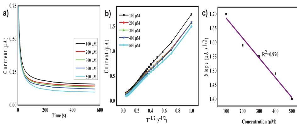
**Figure 8.** Chronoamperometric of the modified electrode in different dopamine concentrations (a) linear plot of current versus time. b) Corresponding current versus  $T^{-1/2}$ . c) Plot of corresponding slopes versus dopamine concentration.
