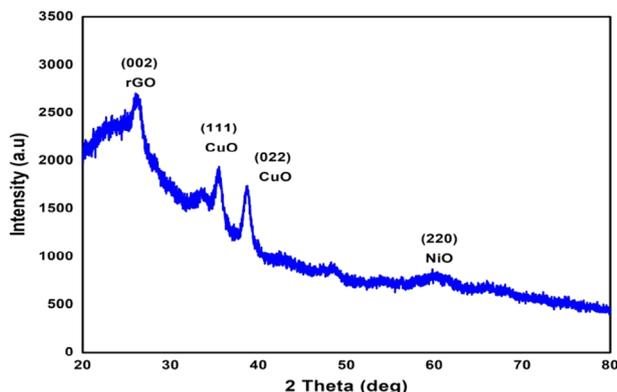
Figure 2. XRD pattern of CuO-NiO/rGO nanocomposite.
