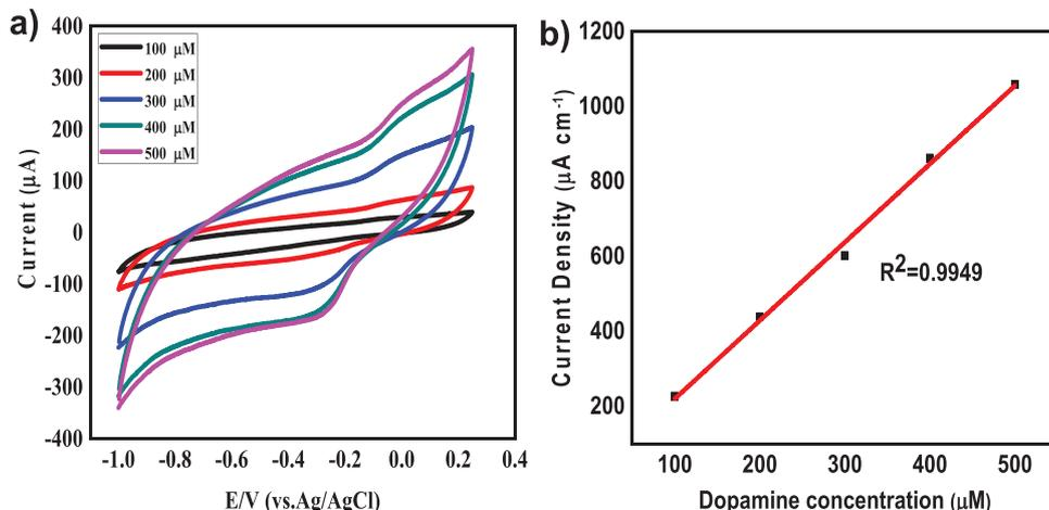
**Figure 6.** a) The linear increase in the anodic and cathodic peak current with the increasing concentration demonstrates the sensitivity of the metal oxide nanocomposite in detecting dopamine.<sup>[32]</sup> b) Linear response of CuO-NiO/rGO nanocomposite with increasing dopamine concentration.
