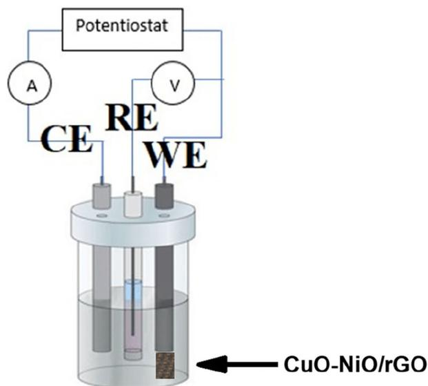
Figure 1. Schematic of electrochemical cell.
