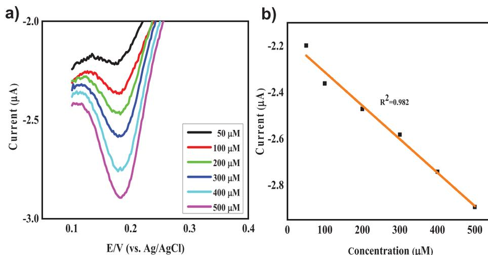
**Figure 9.** Differential pulse voltammetry of the modified electrode in different dopamine concentrations. a) Linear plot of peak current and dopamine concentration. b) Linear regression response of different dopamine concentrations.
