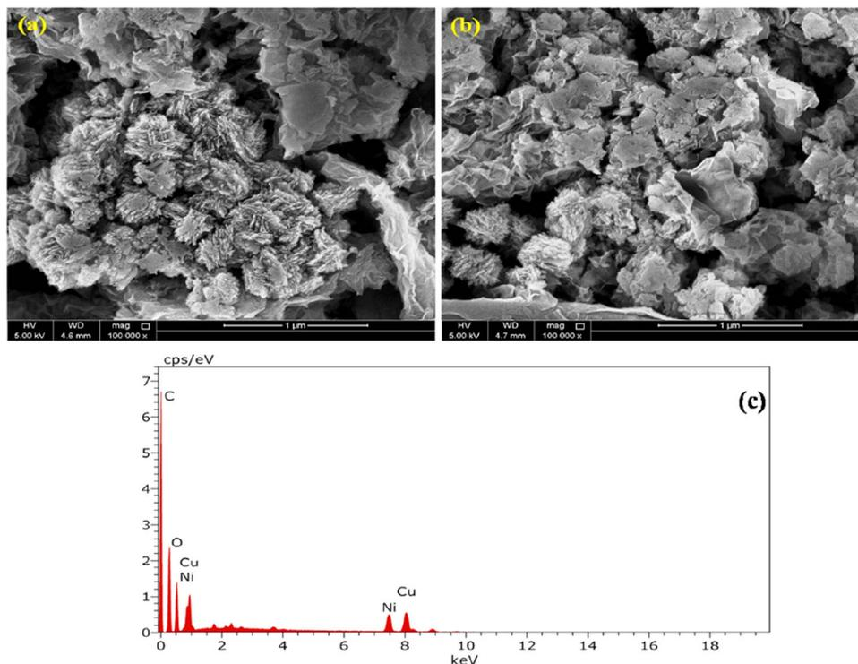
Figure 4. a, b) FE-SEM and (c) EDS images of the prepared nanocomposite.
