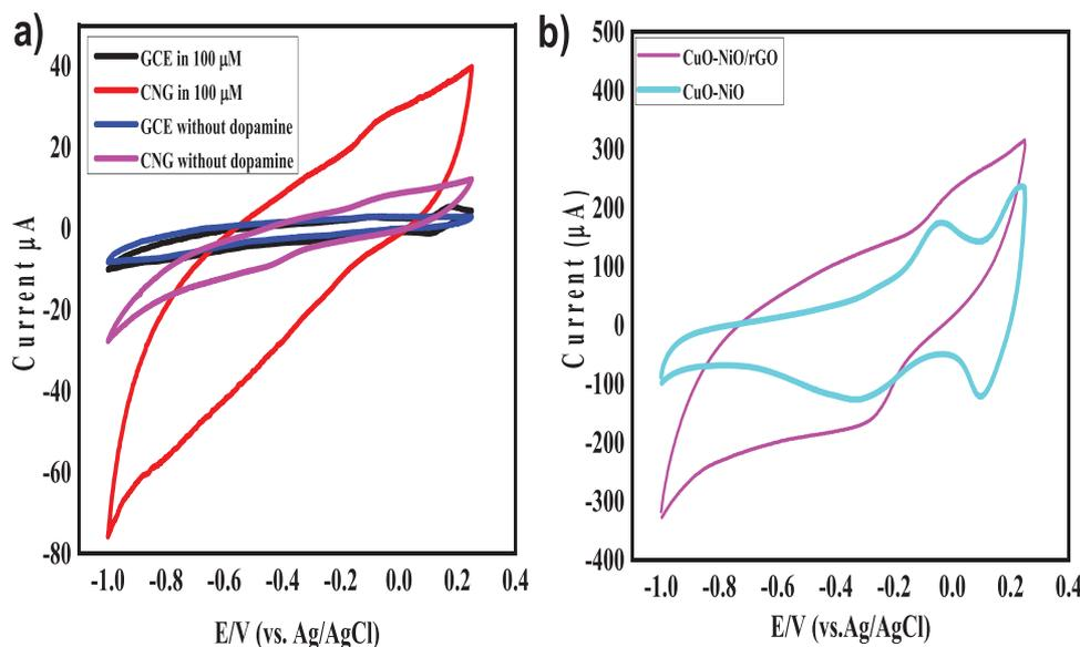
Figure 5. a) Response of bare and modified CuO-NiO/rGO (CNG) with GCE electrodes in the presence and absence of dopamine at  $50 \text{ mV s}^{-1}$  scan rate and b) dopamine ( $500 \mu\text{M}$ ) detection of CuO-NiO nanocomposite with and without rGO at  $50 \text{ mV s}^{-1}$  scan rate.
