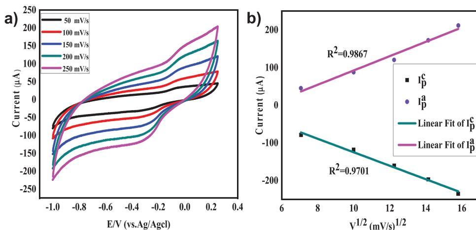
**Figure 7.** a) Electrochemical response of CuO-NiO/rGO with increasing scan rate in 100 μM of dopamine and b) linear regression response of the cathodic and anodic peak currents with a calibration plot.
