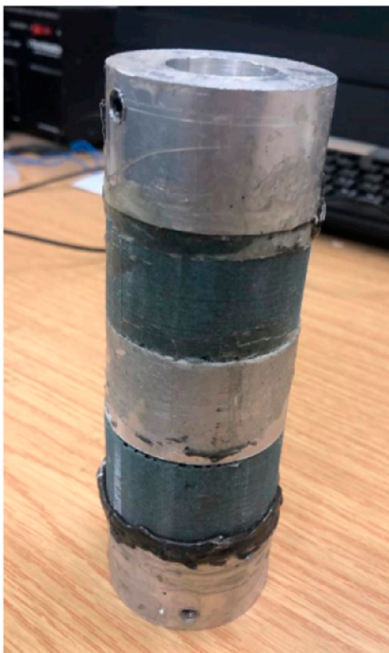
Figure 10. Flexible coupling with MRE. The methodology of the impact hammers test: (a) impact and response locations, (b) input excitation representation and (c) output response representation.
