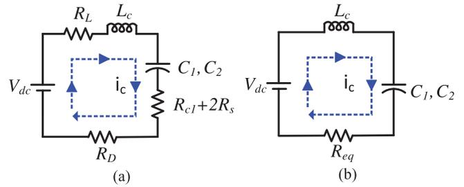
**FIGURE 4** (a) Charging path of the capacitors,  $C_1$  and  $C_2$  (b) Equivalent circuit of charging path of capacitors,  $C_1$  and  $C_2$ .
