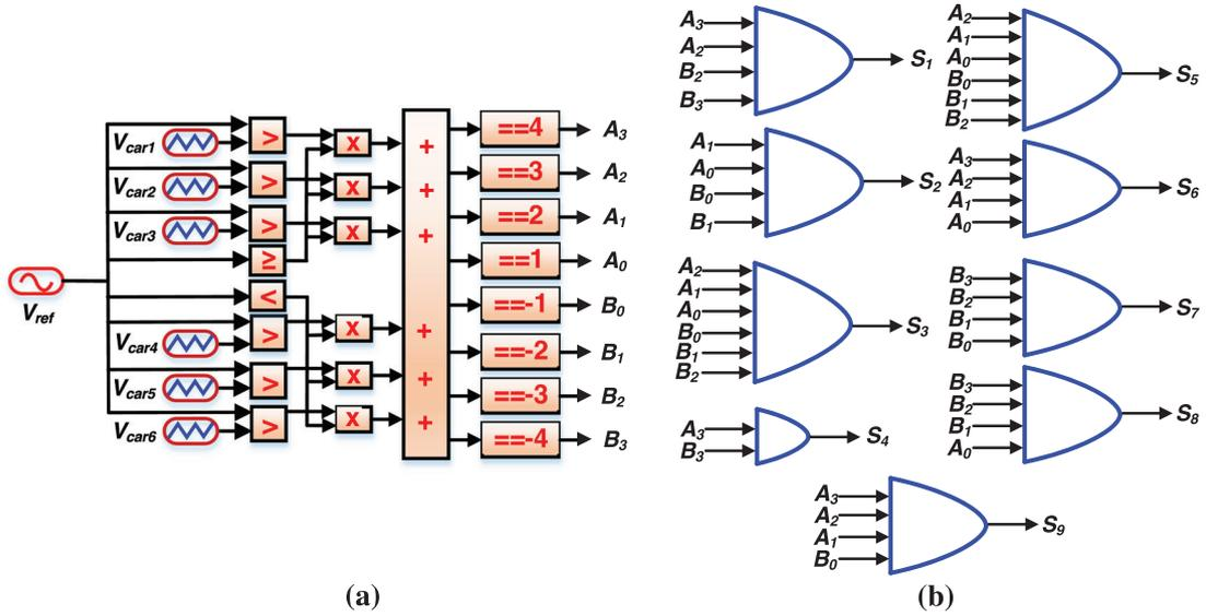
FIGURE 5 (a) Switching scheme of the proposed 7L TB-SCMLI (b) OR logic used to generate gating pulses to switches.
