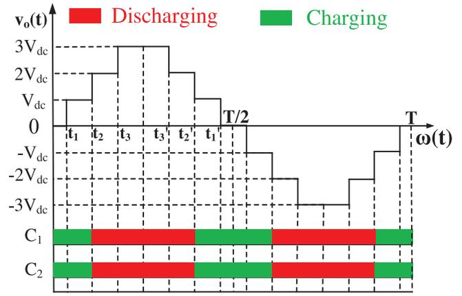
**FIGURE 3** Operating states of the proposed 7L TB-SCMLI at the positive levels.
