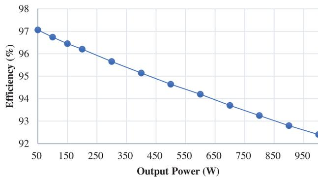
**FIGURE 7** Efficiency curve of the proposed TB-SCMLI topology.
