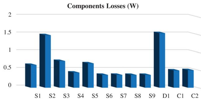
**FIGURE 6** Power loss distribution for the input voltage of 100 V and at an output power of 200 W.
