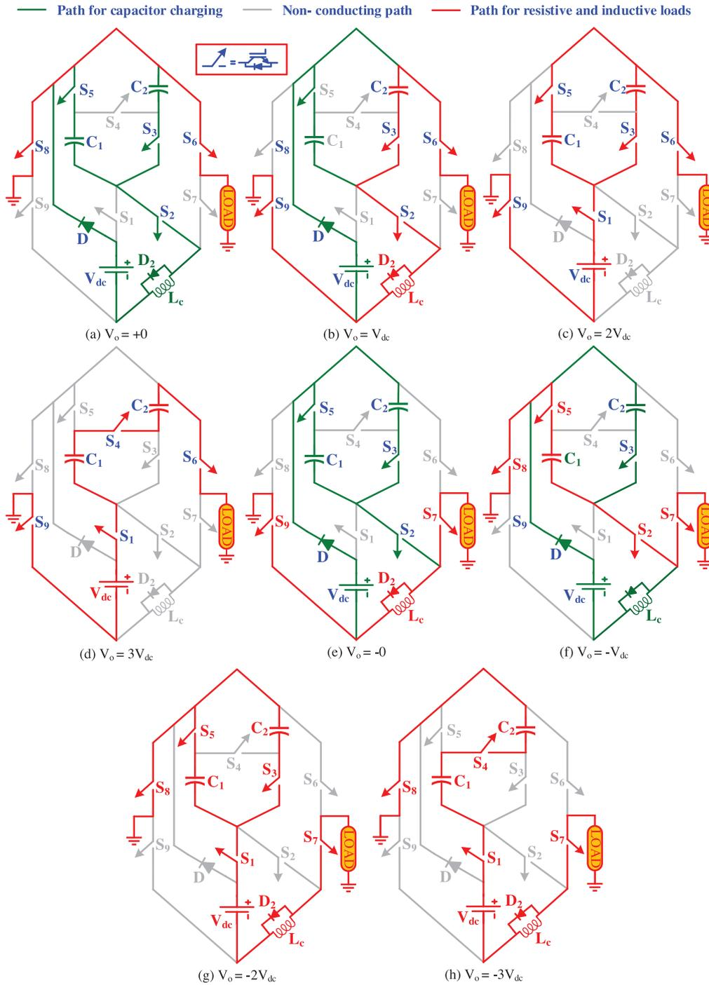
**FIGURE 2** Operating states of the proposed 7L TB-SCMLI at the positive levels.
