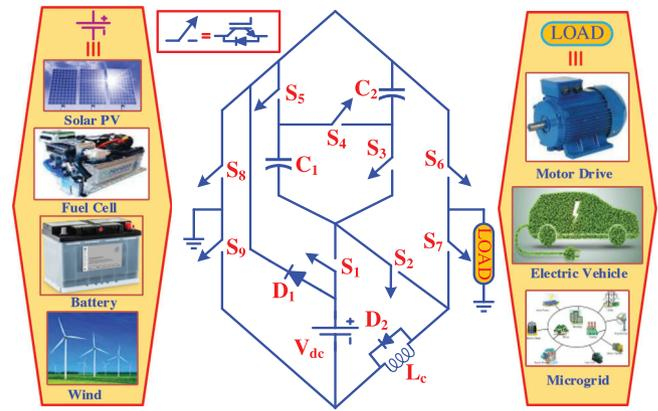
FIGURE 1 Topology configuration of the proposed TB-SCMLI.
