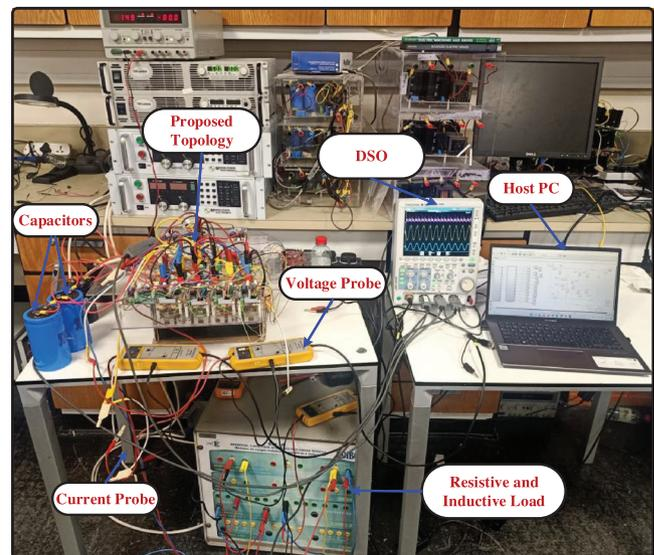
**FIGURE 8** Experimental setup for the proposed TB-SCMLI topology.
