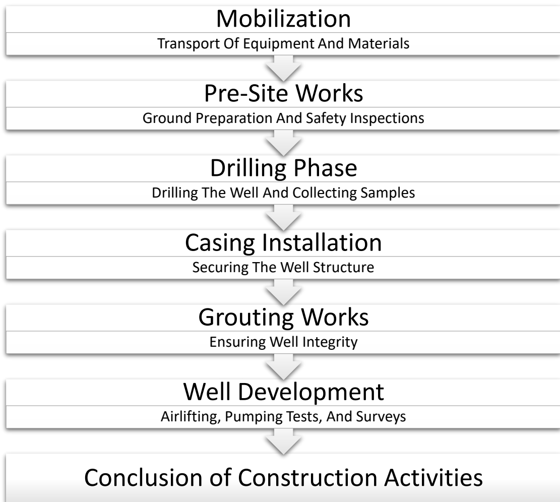
Figure 11. Construction full process.
