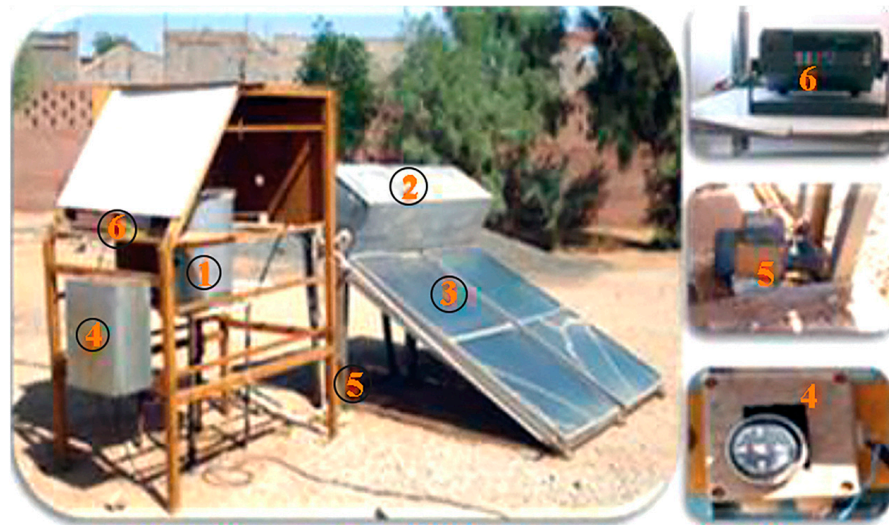
Figure 7. Solar Batch Fermenter: (1) fermenter, (2) water tank, (3) solar heater, (4) control panel, (5) pump, (6) data logger, reprinted from [41].
