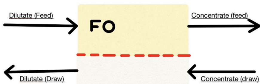
Figure 6. Forward osmosis process principle.
