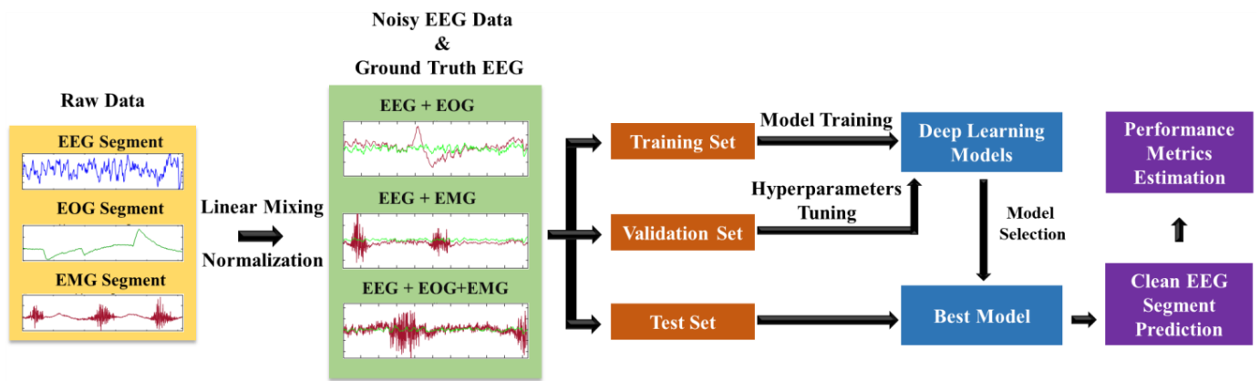
Figure 1. Proposed framework for removing physiological artifacts from EEG signals.
