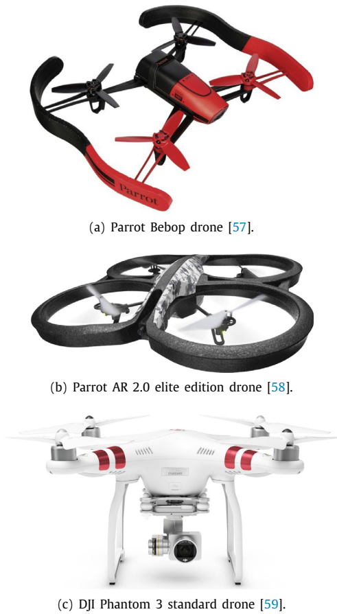
Fig. 2. Three drones used to build the drone RF database.
