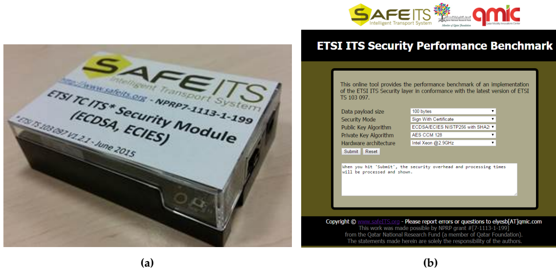
Figure 9. ETSI TC ITS Security Standard Compliant Experimental Test-Bed and Online Tool. (a) ETSI TC ITS Compliant Security Module (BeagleBone version); (b) Online tool for ITS Security Performance Benchmark [18].
