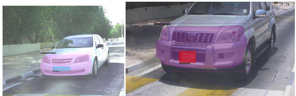
Figure 9. Resultant images of segmentation and classification using the maskRCNN with the Resnet-50 backbone.
