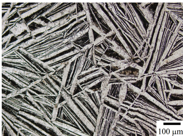
Fig. 6 – Microstructure images for induction melted \text{Bi}_2\text{Te}_{2.55}\text{Se}_{0.45} disc.
