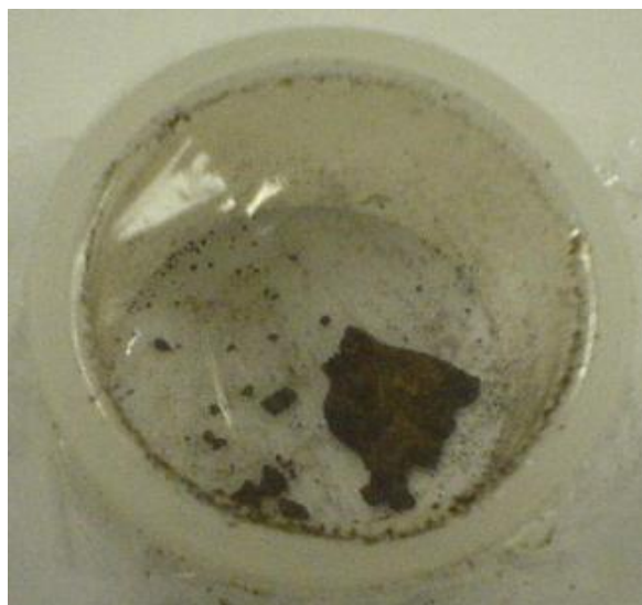
Figure 4. Corrosion products taken from inside the T-joint
