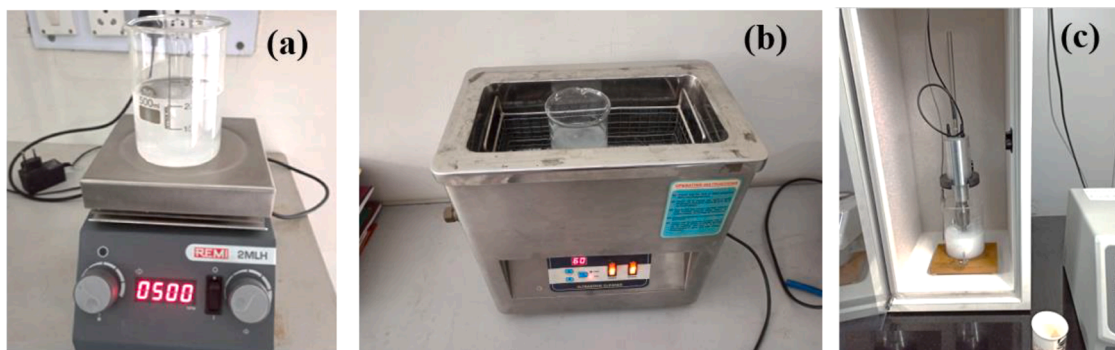
Fig. 4. (a) Magnetic stirring with heating (b) bath sonication with heating (c) Sonication with probe sonicator.
