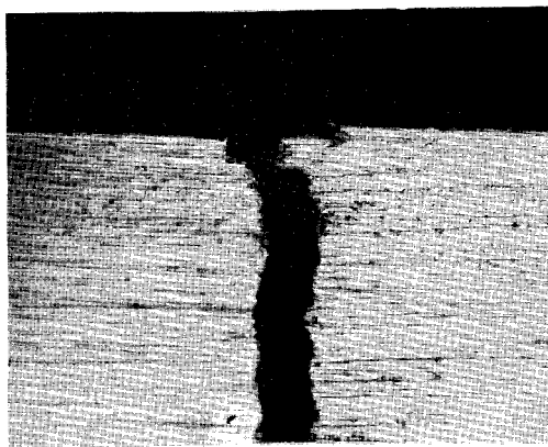
Figure 5: Crack Initiation at 45° to the Surface (Grit 600 and 500x).
