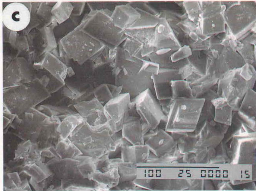
Fig. 3: A- Polish slab of the laminated dolomite (L), the dolomite matrix (M), and the dolomite intraclasts (I). B- Photomicrograph of breccia of microfabric dolomite. Note the difference in size and shape of the crystals between the dolomite intraclasts and the dolomite matrix. C- SEM image of dolomite matrix crystals. D- Numerous thin zones which range from brightly luminescent to non-luminescent and characterize the dolomite intraclasts type.
