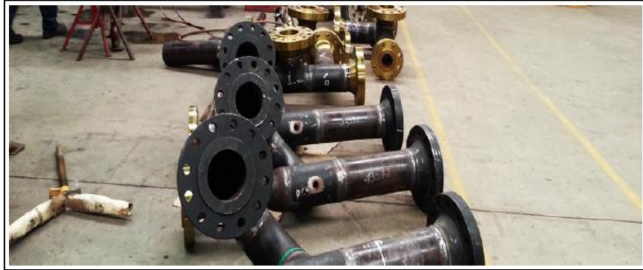
Figure 27. Sample of tack weld spools
