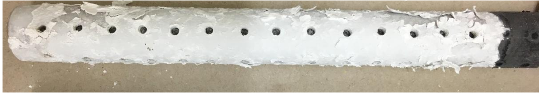
Figure 31: Cathode passivation after 90 minutes of continuous operation
