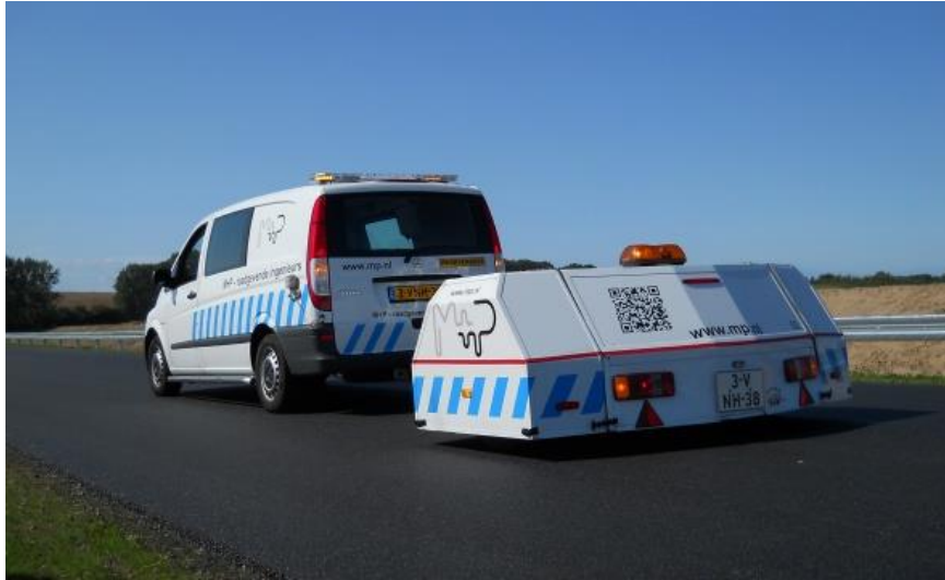
Figure 4. CPX trailer manufactured by M+P (Source: www.mplusp.eu )
