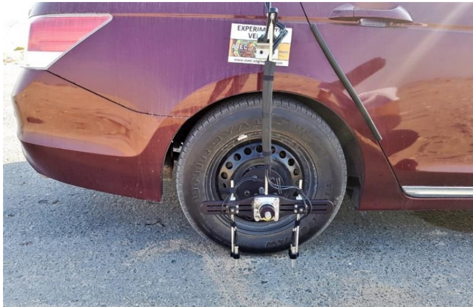
Figure 10. Mounted OBSI testing rig
