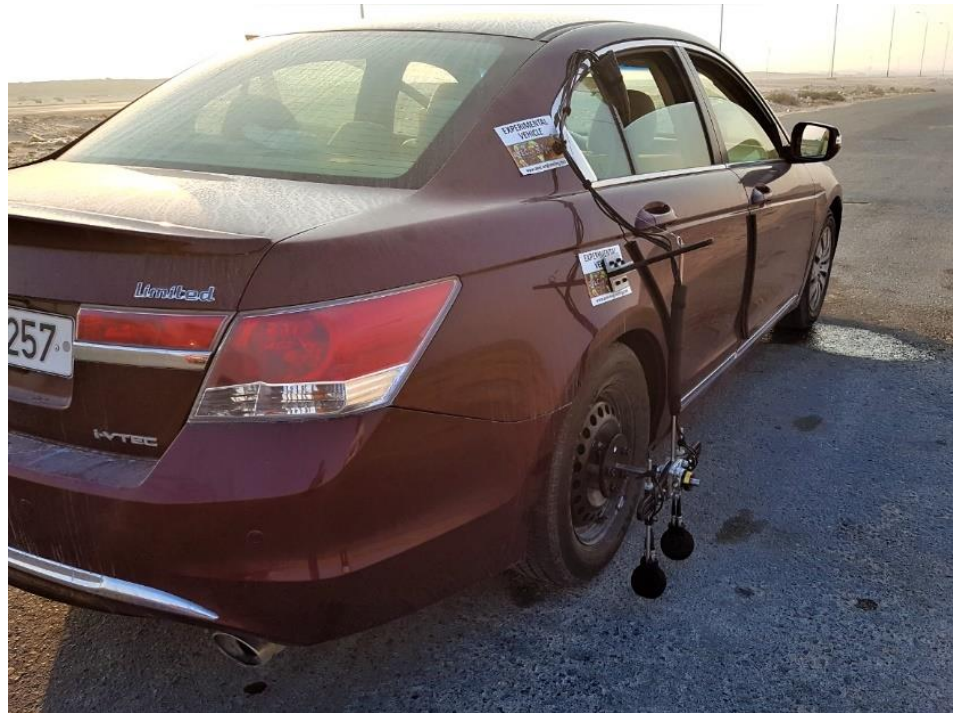
Figure 6. OBSI testing equipment
