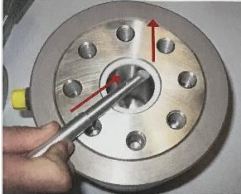
Figure 3-4: The liquid sample cylinder where the magnetic stirrer is located
