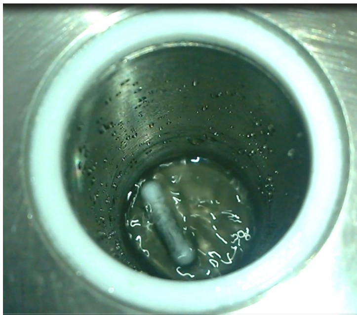
Figure 3-5: Magnetic stirrer inside the high-pressure cell that is agitated using the lab mixture placed below the high-pressure cell.
