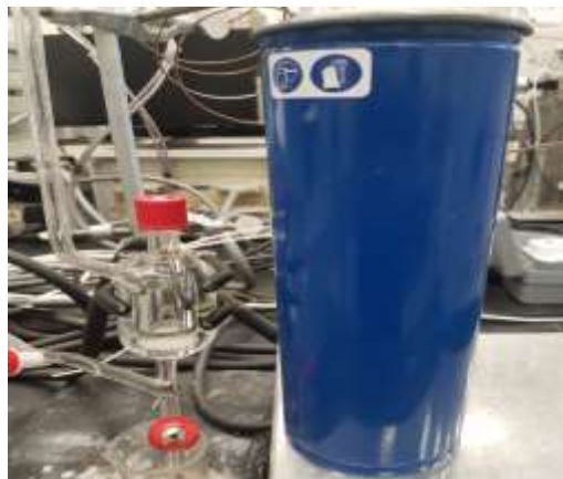
C) Sample injecting vessel and Dry ice Trap
