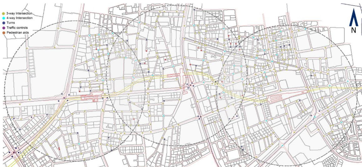
Figure 60. Intersection density calculated using 3/4-way intersections, turns and traffic controls for Bin Mahmoud, Al Sadd and Joaan (Source: Author,2018)
