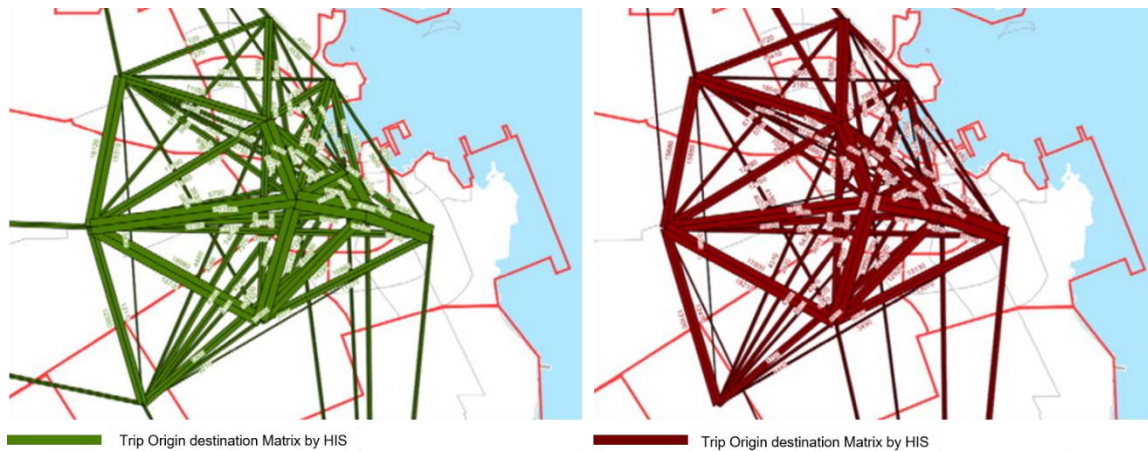
Figure 3. Clustered O-D matrix obtained using HIS and VISUM model (Source: Hamra & Attallah, 2012)
