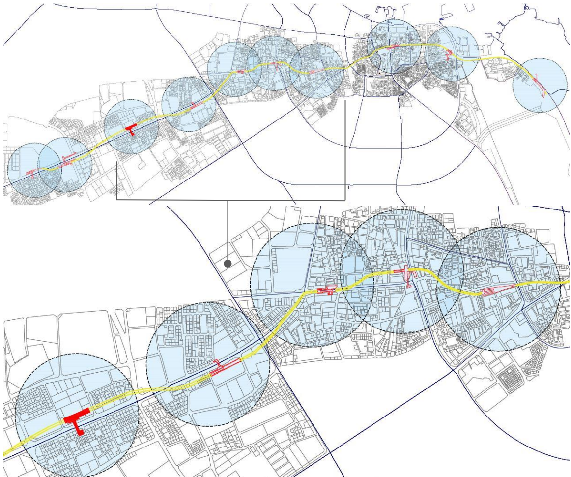
Figure 33. Defining the catchment area of metro stations within 700m radius – 5min. walking distance (Source: Author, 2018)
