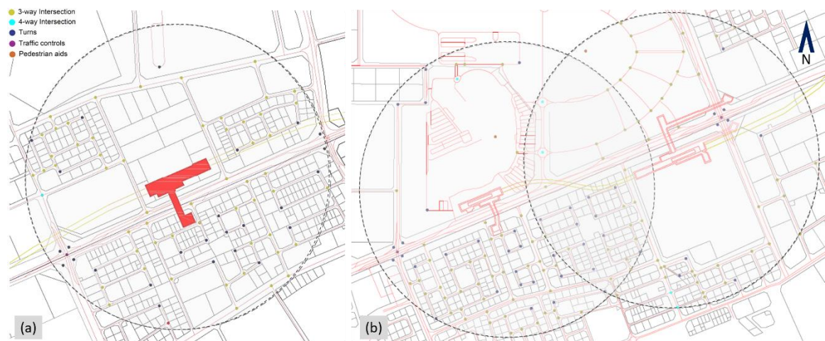
Figure 59. Intersection density calculated using 3/4-way intersections, turns and traffic controls for (a) Al Waab, (b) Sports City and Al Aziziyah (Source: Author,2018)
