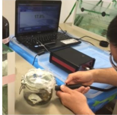
Figure 7: Arrangement of Pinctada radiata into individual jars (top pictures) for measuring oxygen concentrations using the OxySense platform (bottom pictures)
