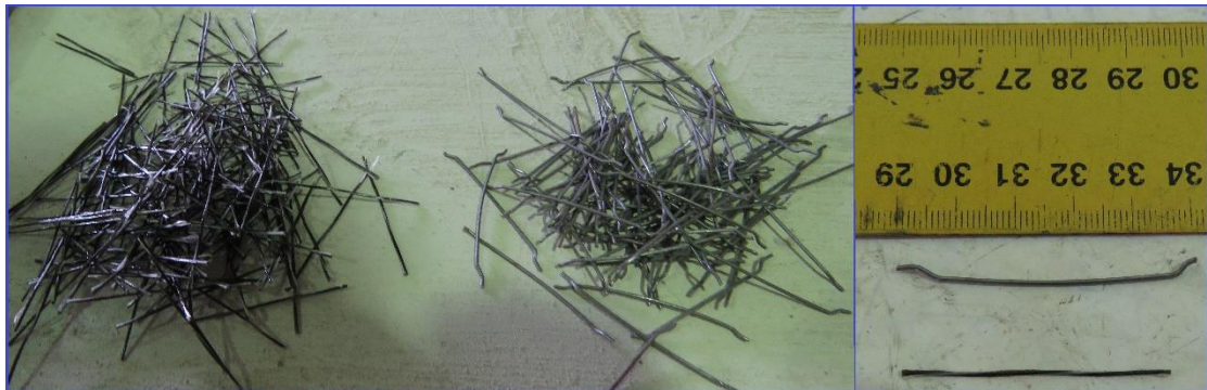
Figure 22: Steel and Basalt Fibers Used in this Study.
