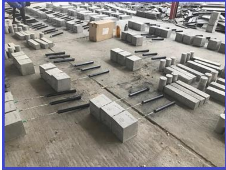
Figure 23: Pullout Specimens after Curing.
