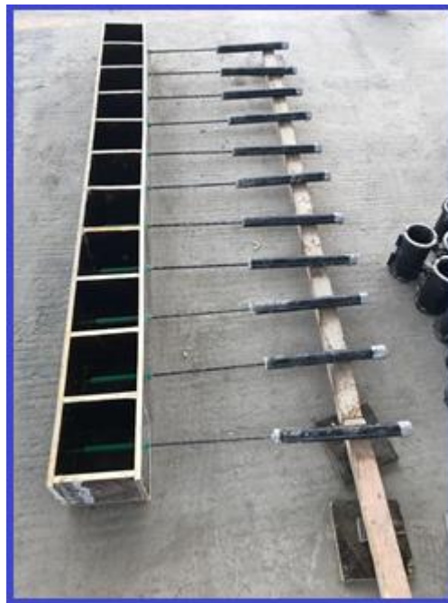
Figure 24: Plywood Molds Used for Casting Pullouts Specimens.
