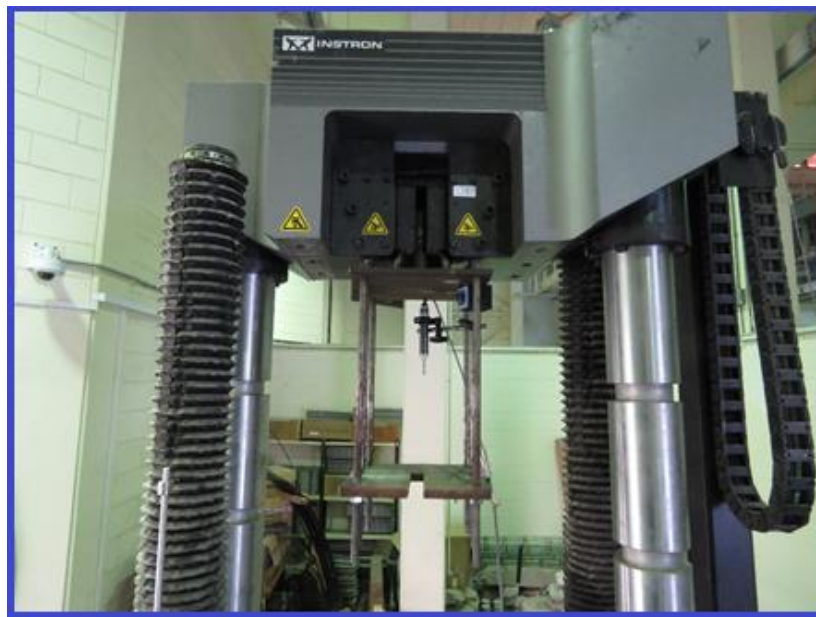
Figure 29: Fabricated Pullout Steel Frame Setup.
