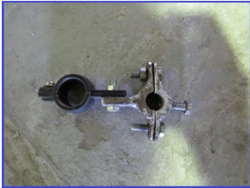
Figure 31: Fabricated Steel Bracket Used to Hold the Bottom LVDT.
