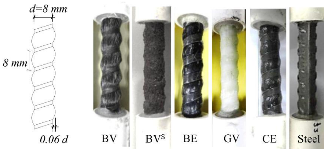
Figure 15:FRP Bars Tested in [61]
