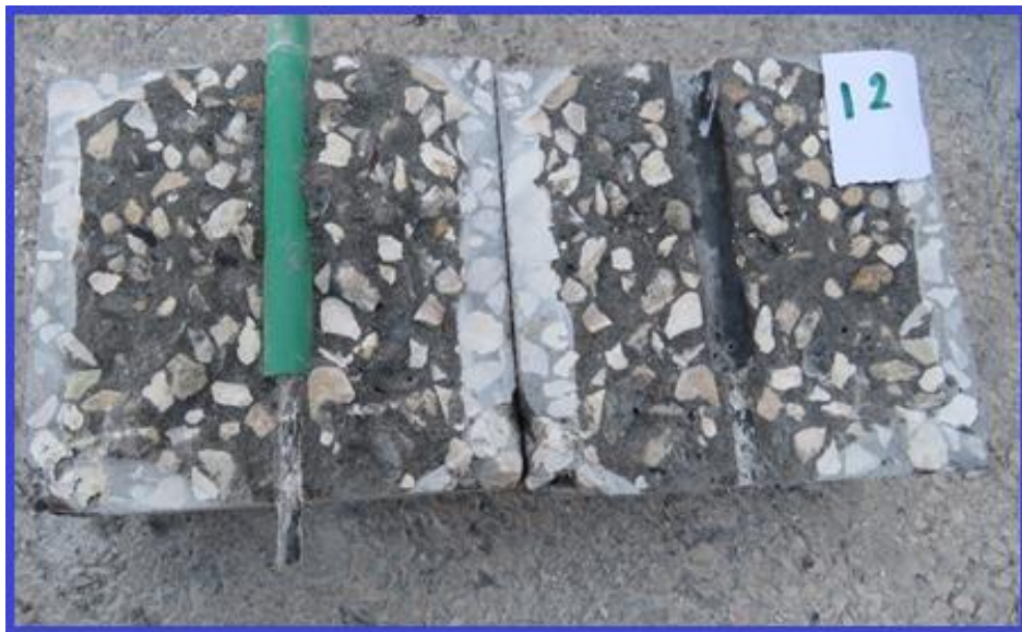
Figure 39: Closer Examination of conditioned Plain Concrete after 90 Days at 35 °C .
