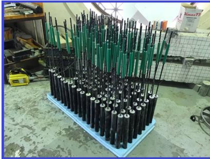
Figure 27: Bar Preparation before Casting.
