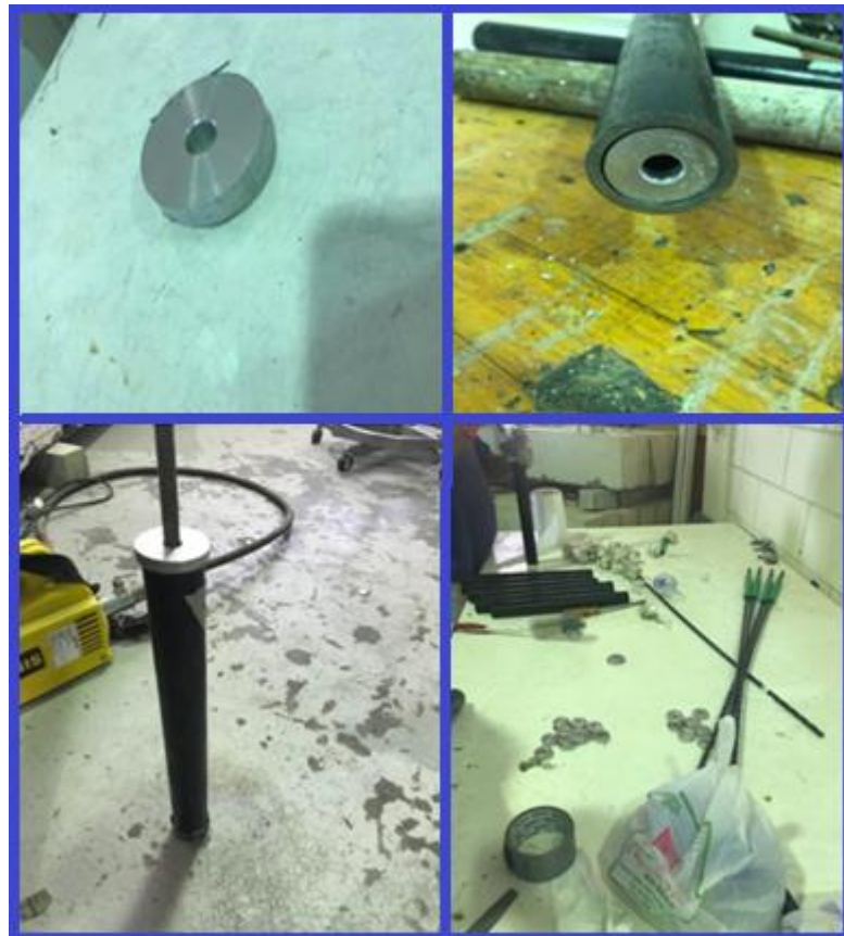
Figure 26: Washers Fabricated to Centralize the Bar inside the Steel Tube.
