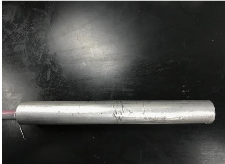
Figure 5. Symmetrical aluminum inner electrode for AC/DC.
