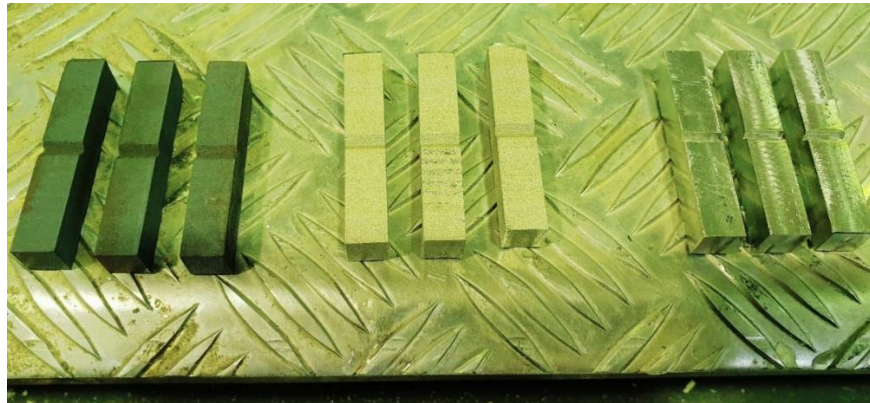
Figure 17: Fabricated impact samples ready for testing right to left: CNC machined, As built 3D printed & Heat treated 3D printed
