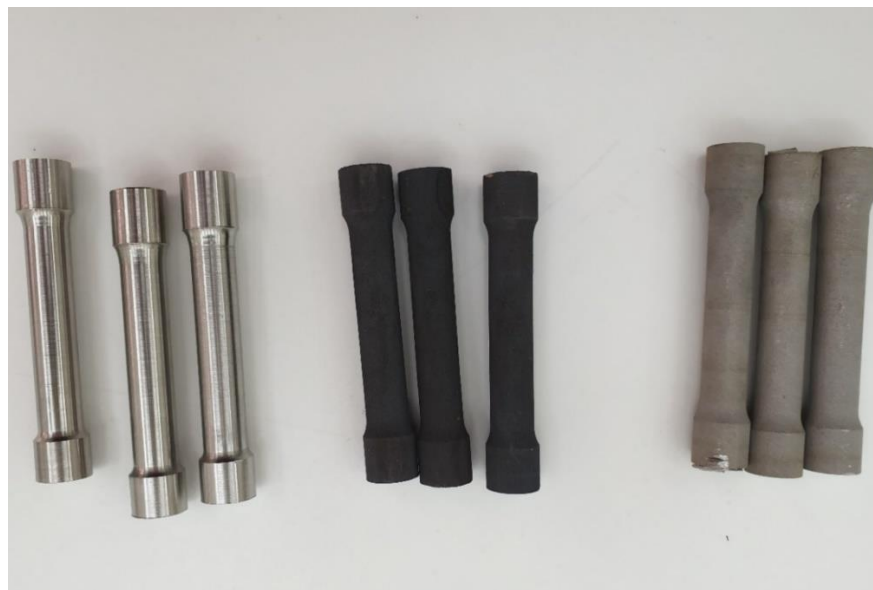
Figure 16: Fabricated tensile samples ready for testing right to left: As built 3D printed, Heat treated 3D printed & CNC machined
