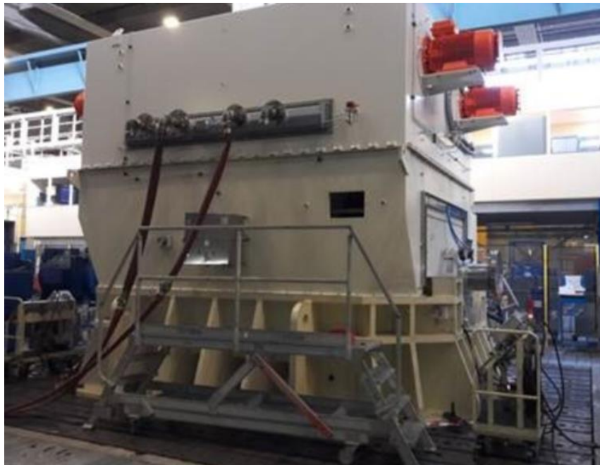
Figure 2-3 Largest 80MW induction motor during no-load test.
