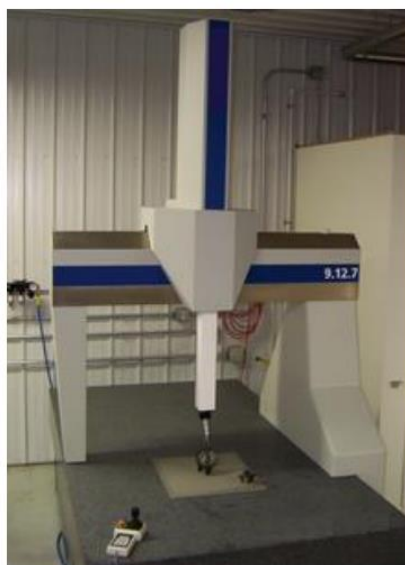
Figure 30. Coordinate Measuring Machine (CMM) (Mostafa A-B Ebrahim, 2014)
