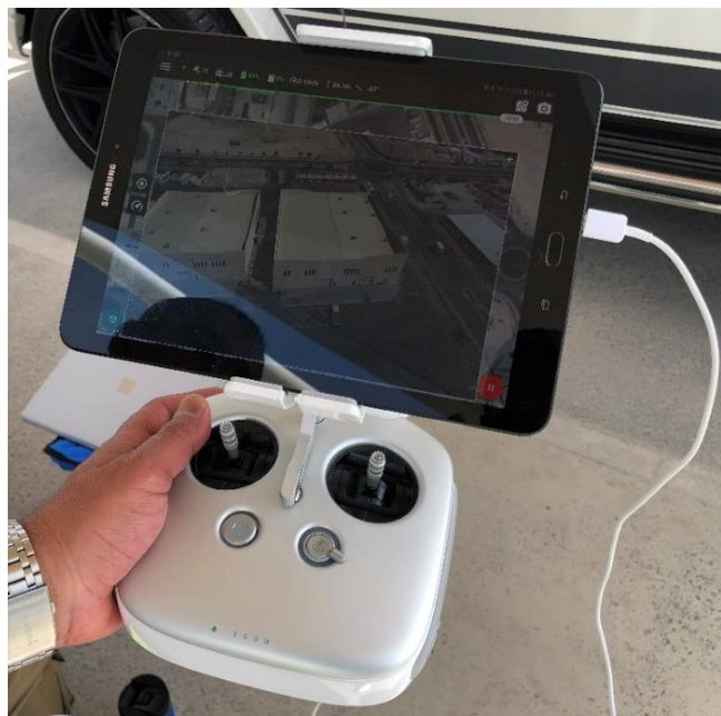
Figure 104. Adjusting and reviewing project mission through DroneDeploy app
