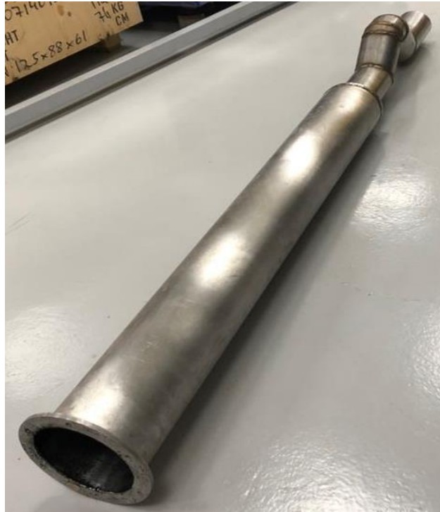
Figure 30. Emissions reduction pipe
