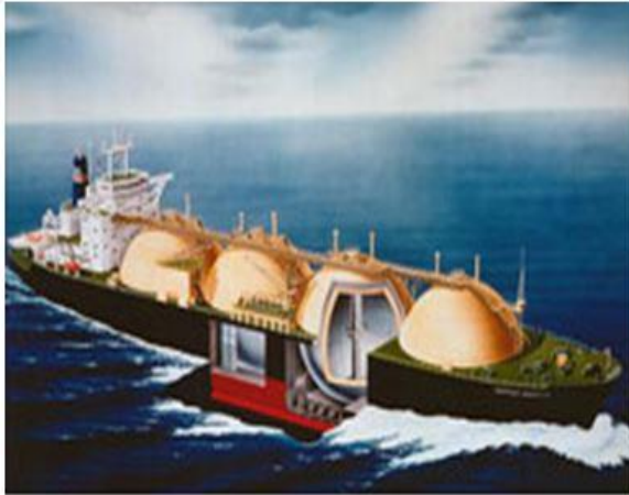
Section through Moss LNG vessel
