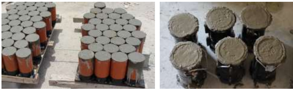
Figure 13: Batch A specimens (a) Initial Curing; (b)Control Specimens
