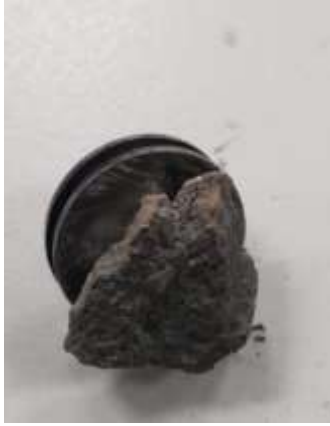
Figure 16: Gold Plated Sample for SEM analysis
