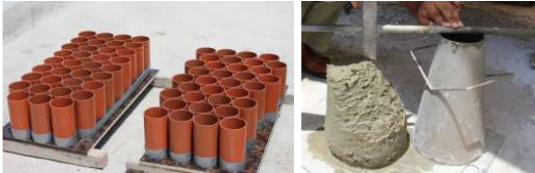
Figure 10: (a) Moulds for Casting; (b) Slump Test
