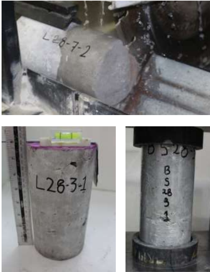
Figure 15: Compressive strength test procedure
