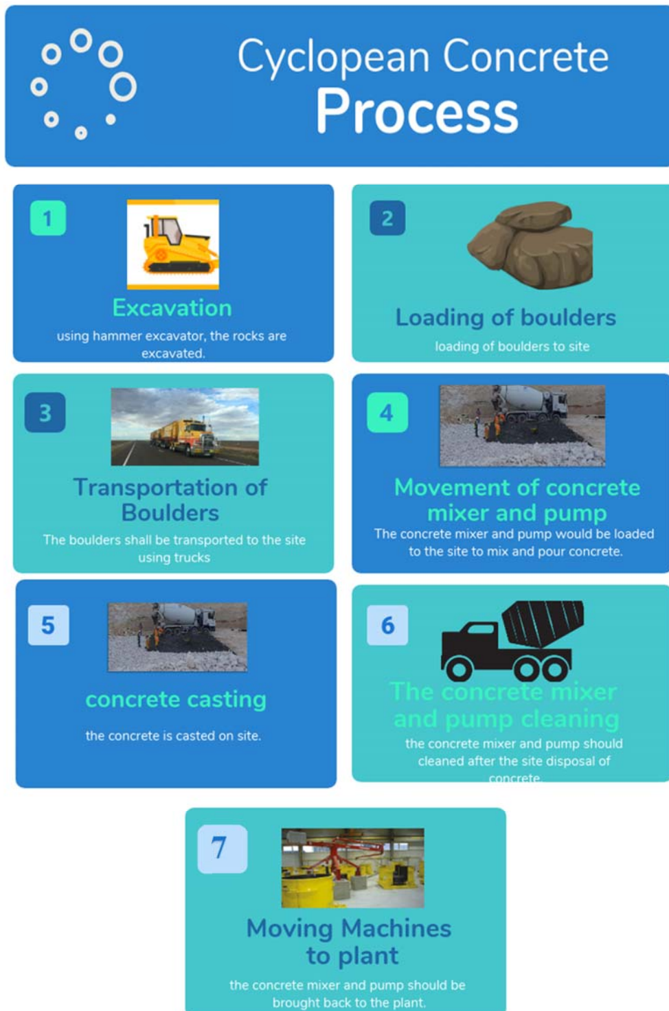
Figure 7: illustrates the flow process using Cyclopean Concrete
